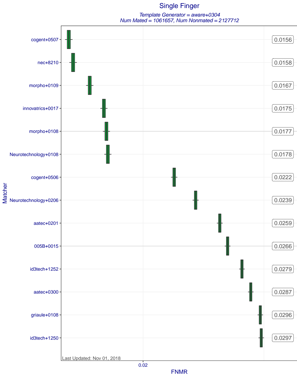
Figure 5: Single Finger FNMRs at FMR=0.0001 when MINEX III compliant matchers compare templates created by template generator aware+0304. Each box represents uncertainty about the true FNMR. The box edges mark the 50% confidence intervals while the whiskers mark the 90% confidence intervals. The numbers on the right show the actual computed FNMRs.
