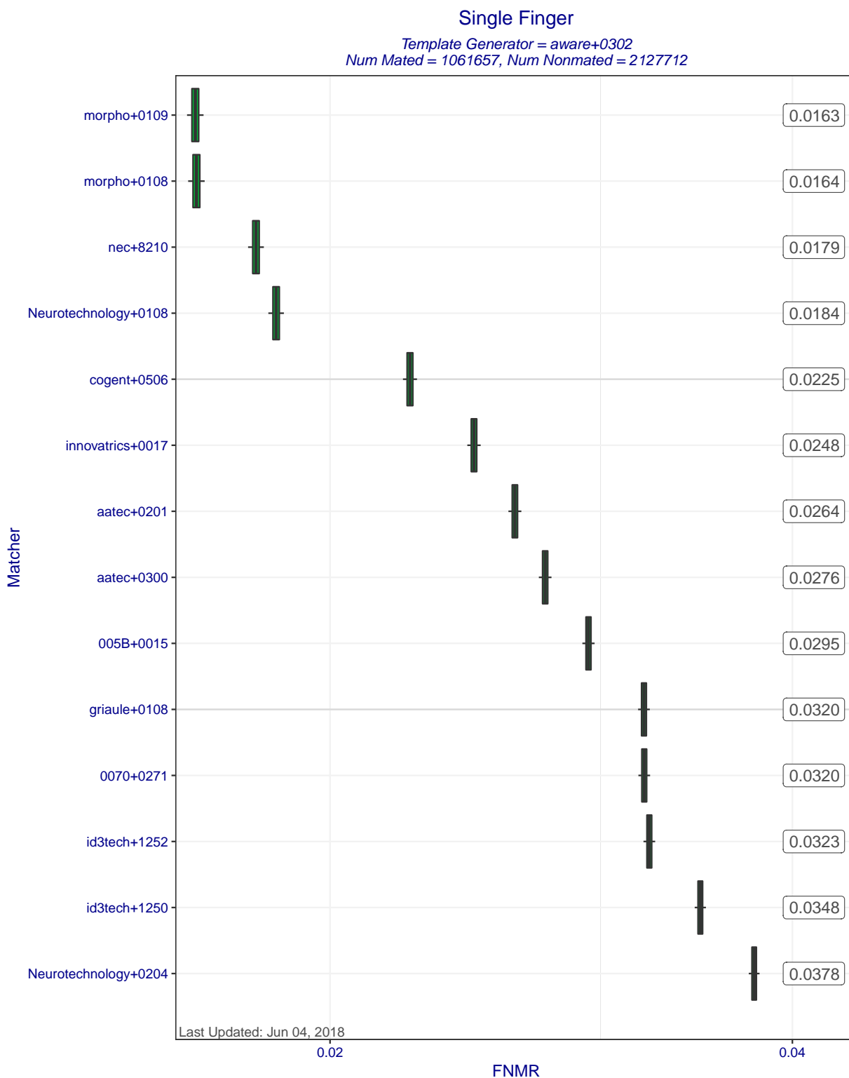
Figure 5: Single Finger FNMRs at FMR=0.0001 when MINEX III compliant matchers compare templates created by template generator aware+0302. Each box represents uncertainty about the true FNMR. The box edges mark the 50% confidence intervals while the whiskers mark the 90% confidence intervals. The numbers on the right show the actual computed FNMRs.
