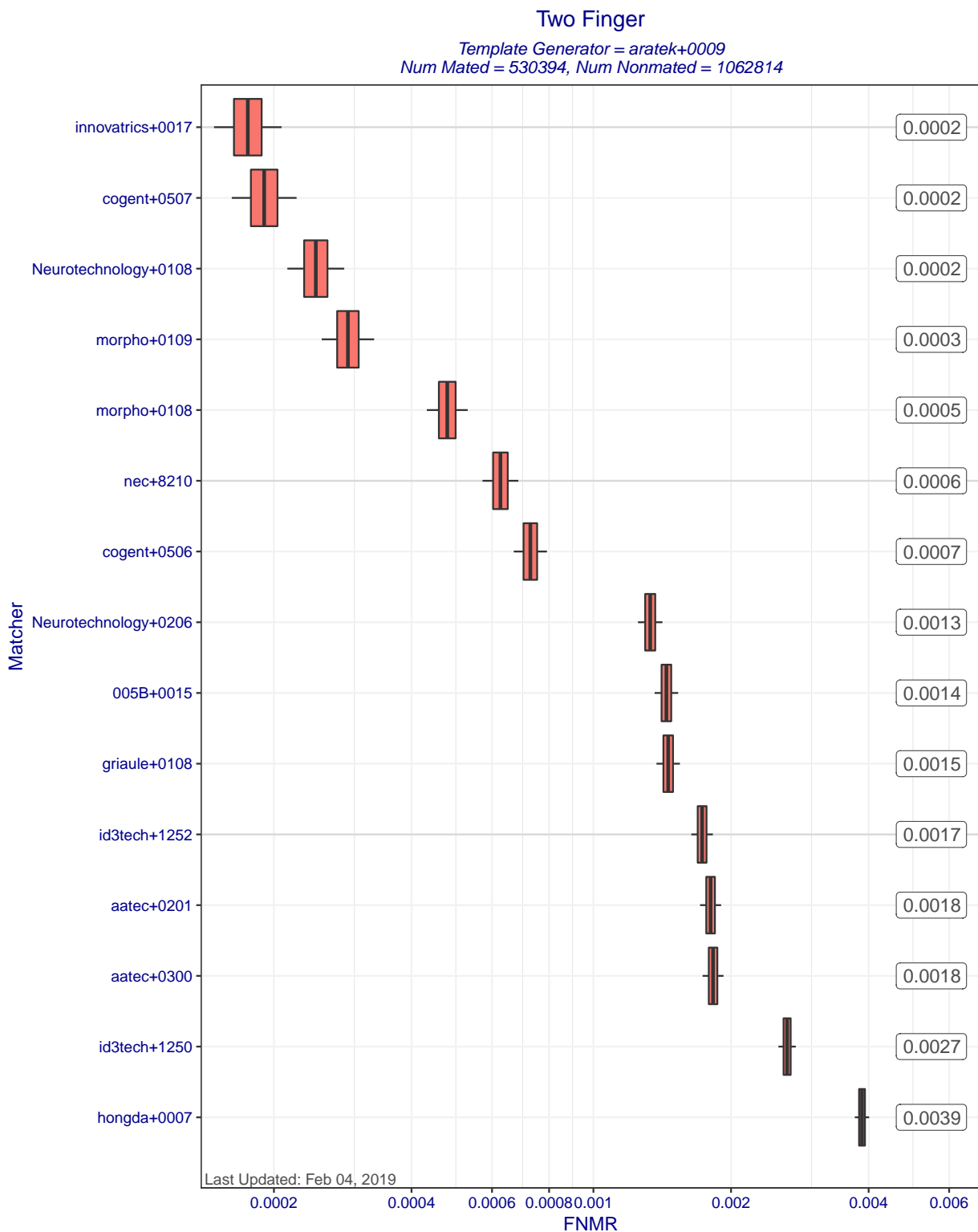
Figure 7: Two Finger FNMR at FMR=0.01 when different matchers compare templates created by template generator aratek+0009. Each box represents uncertainty about the true FNMR. The box edges mark the 50% confidence intervals while the whiskers mark the 90% confidence intervals. The numbers on the right show the actual computed FNMRs. Score-level fusion is achieved by averaging the scores for left and right index fingers.
