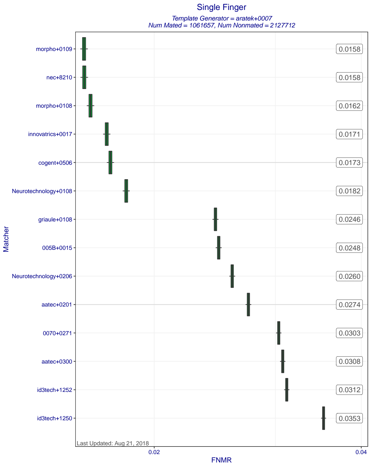
Figure 5: Single Finger FNMRs at FMR=0.0001 when MINEX III compliant matchers compare templates created by template generator aratek+0007. Each box represents uncertainty about the true FNMR. The box edges mark the 50% confidence intervals while the whiskers mark the 90% confidence intervals. The numbers on the right show the actual computed FNMRs.
