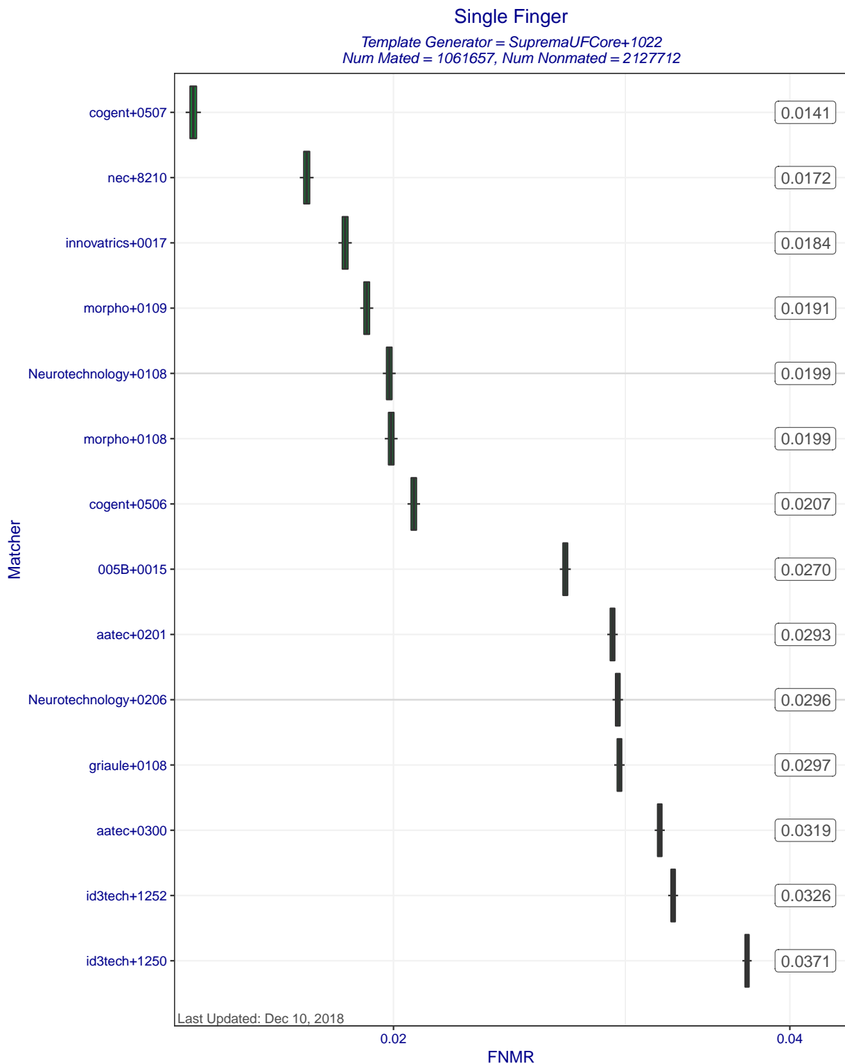
Figure 5: Single Finger FNMRs at FMR=0.0001 when MINEX III compliant matchers compare templates created by template generator SupremaUFCore+1022. Each box represents uncertainty about the true FNMR. The box edges mark the 50% confidence intervals while the whiskers mark the 90% confidence intervals. The numbers on the right show the actual computed FNMRs.
