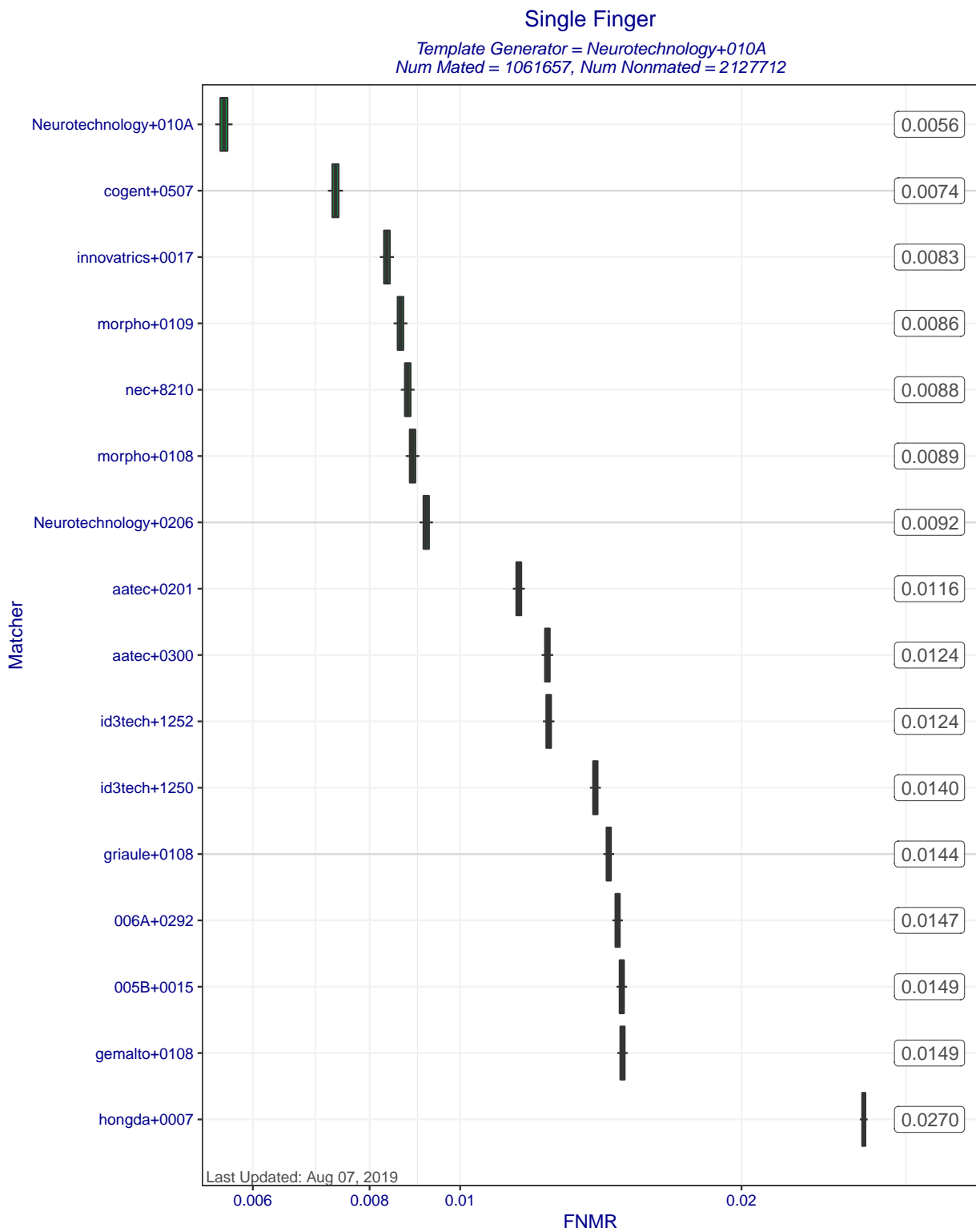
Figure 5: Single Finger FNMRs at FMR=0.0001 when MINEX III compliant matchers compare templates created by template generator Neurotechnology+010A. Each box represents uncertainty about the true FNMR. The box edges mark the 50% confidence intervals while the whiskers mark the 90% confidence intervals. The numbers on the right show the actual computed FNMRs.
