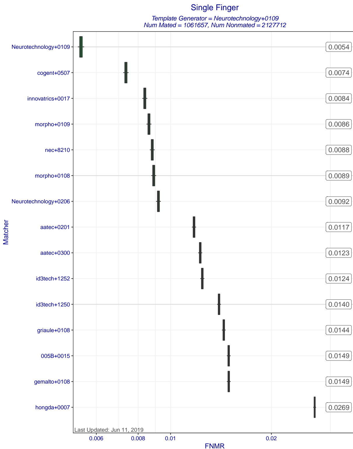
Figure 5: Single Finger FNMRs at FMR=0.0001 when MINEX III compliant matchers compare templates created by template generator Neurotechnology+0109. Each box represents uncertainty about the true FNMR. The box edges mark the 50% confidence intervals while the whiskers mark the 90% confidence intervals. The numbers on the right show the actual computed FNMRs.
