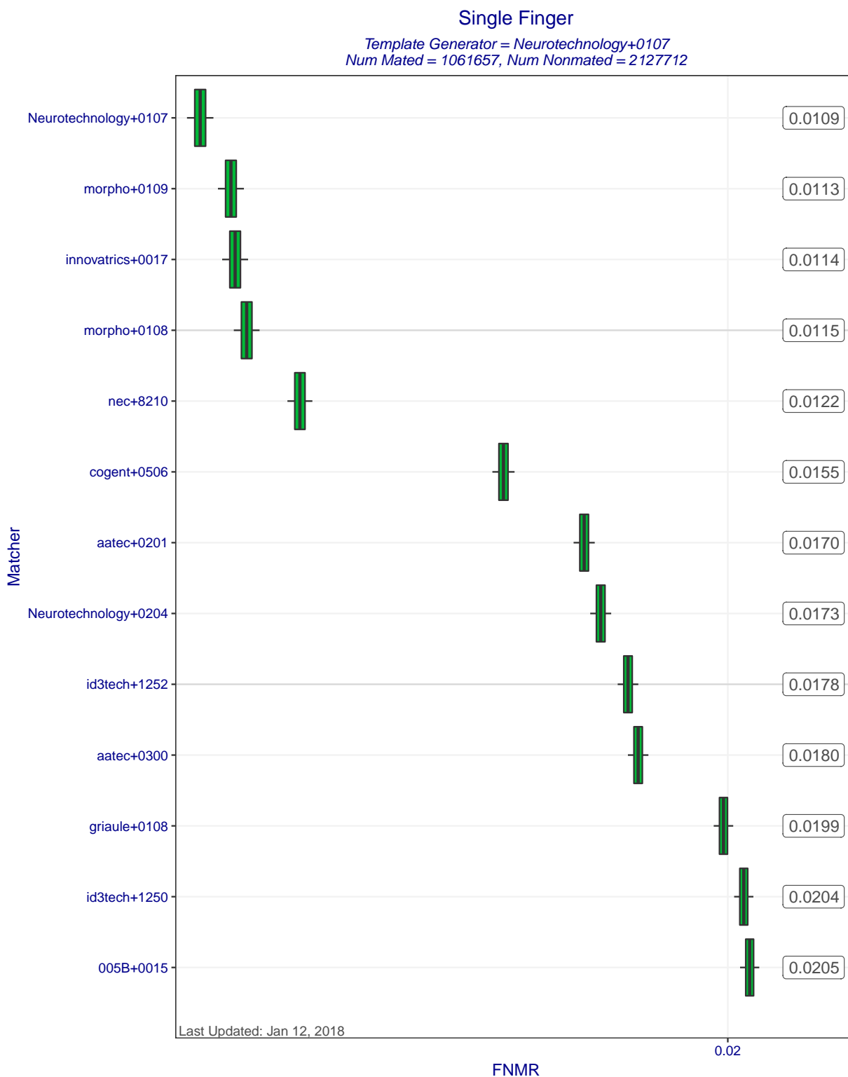
Figure 5: Single Finger FNMRs at FMR=0.0001 when MINEX III compliant matchers compare templates created by template generator Neurotechnology+0107. Each box represents uncertainty about the true FNMR. The box edges mark the 50% confidence intervals while the whiskers mark the 90% confidence intervals. The numbers on the right show the actual computed FNMRs.
