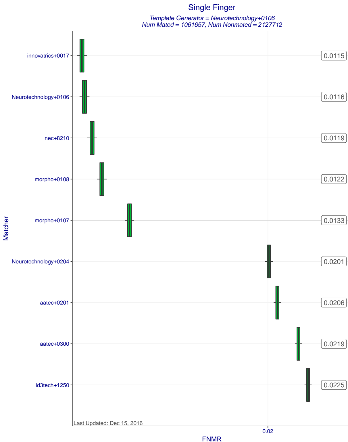
Figure 5: Single Finger FNMRs at FMR=0.0001 when MINEX III compliant matchers compare templates created by template generator Neurotechnology+0106. Each box represents uncertainty about the true FNMR. The box edges mark the 50% confidence intervals while the whiskers mark the 90% confidence intervals. The numbers on the right show the actual computed FNMRs.
