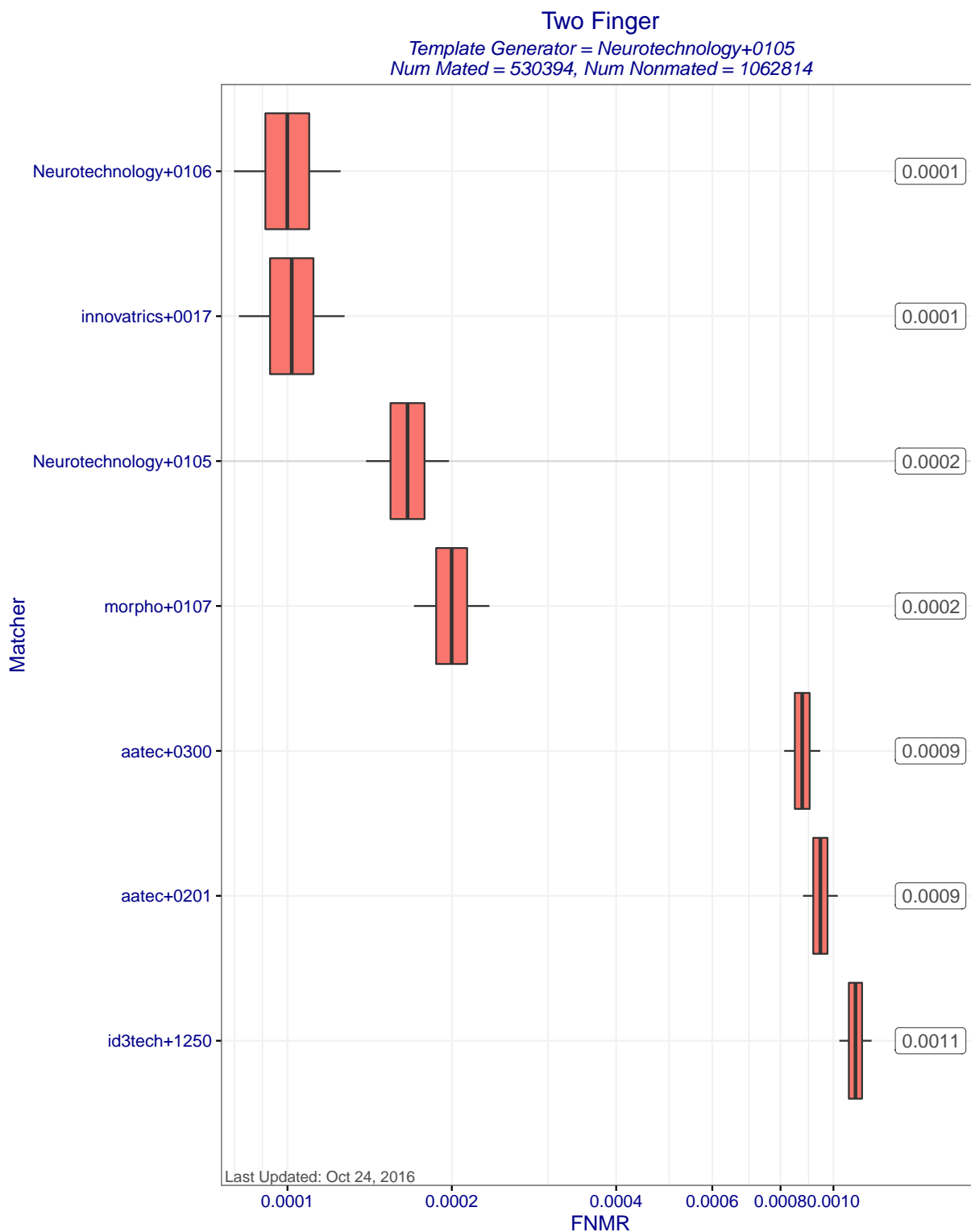
Figure 7: Two Finger FNMR at FMR=0.01 when different matchers compare templates created by template generator Neurotechnology+0105. Each box represents uncertainty about the true FNMR. The box edges mark the 50% confidence intervals while the whiskers mark the 90% confidence intervals. The numbers on the right show the actual computed FNMRs. Score-level fusion is achieved by averaging the scores for left and right index fingers.
