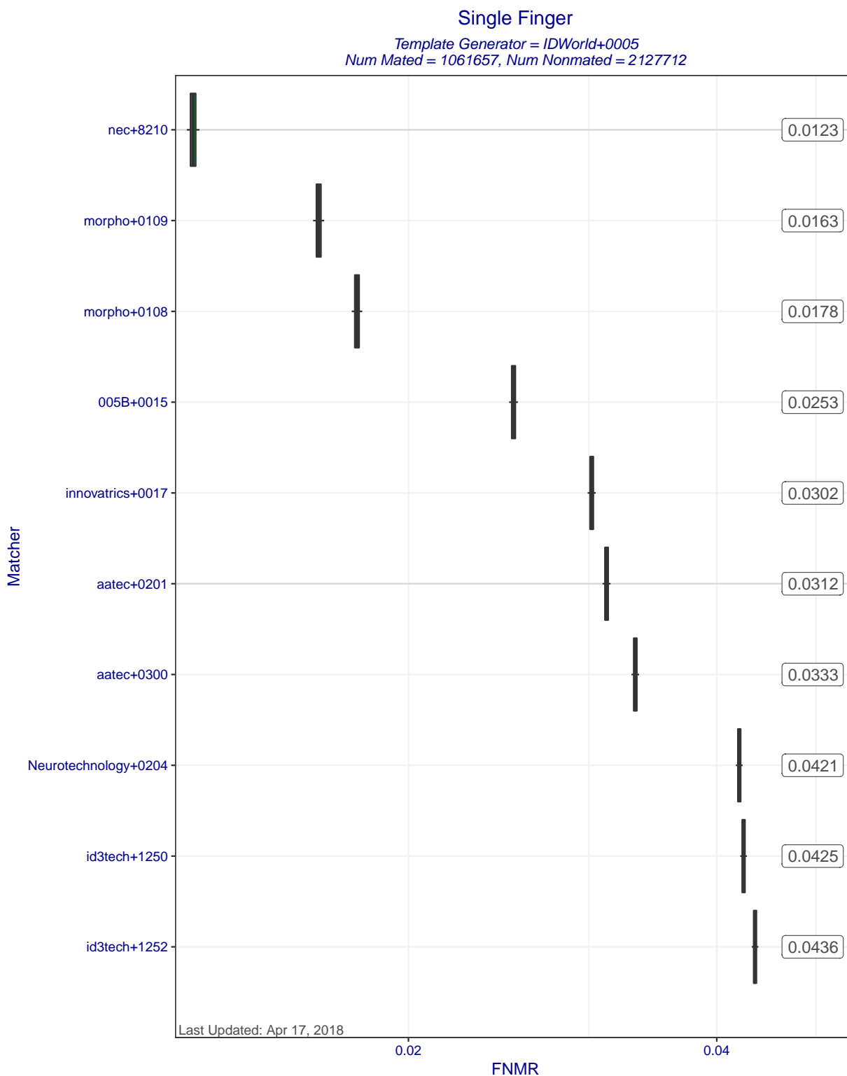
Figure 5: Single Finger FNMRs at FMR=0.0001 when MINEX III compliant matchers compare templates created by template generator IDWorld+0005. Each box represents uncertainty about the true FNMR. The box edges mark the 50% confidence intervals while the whiskers mark the 90% confidence intervals. The numbers on the right show the actual computed FNMRs.
