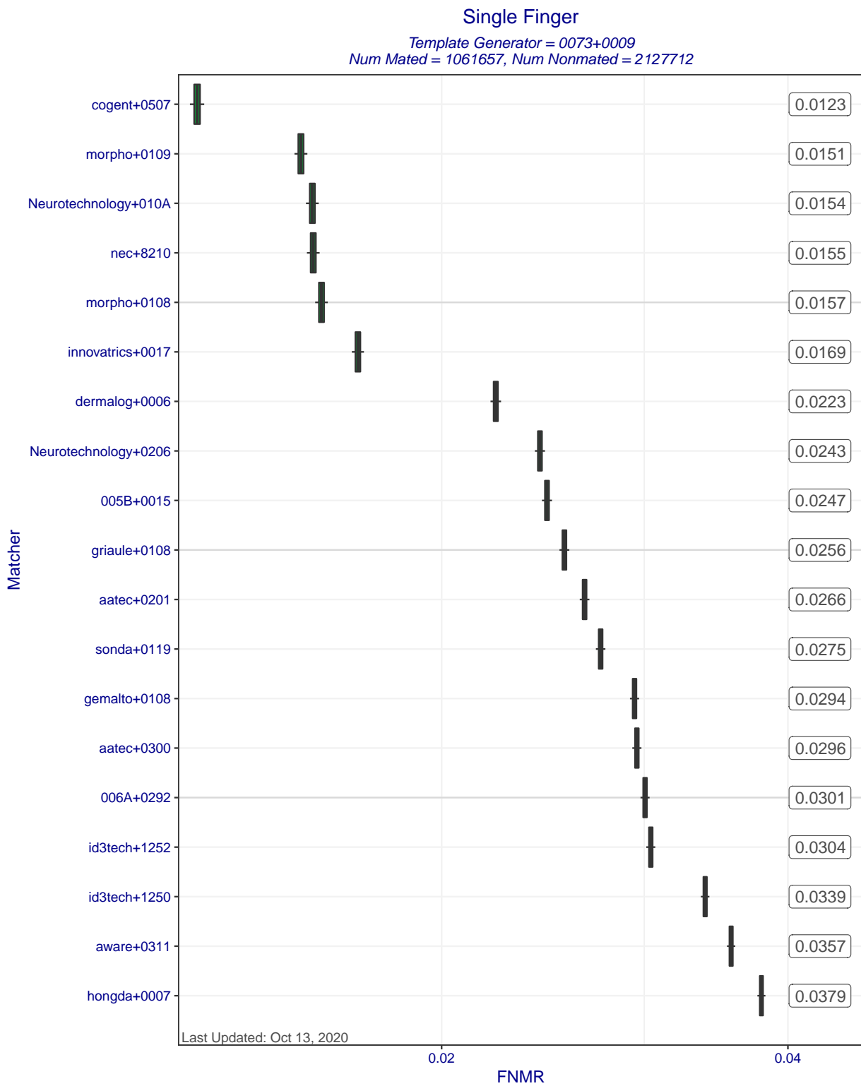
Figure 5: Single Finger FNMRs at FMR=0.0001 when MINEX III compliant matchers compare templates created by template generator 0073+0009. Each box represents uncertainty about the true FNMR. The box edges mark the 50% confidence intervals while the whiskers mark the 90% confidence intervals. The numbers on the right show the actual computed FNMRs.
