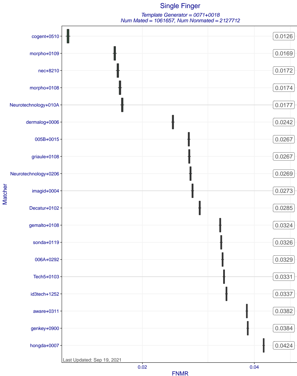
Figure 5: Single Finger FNMRs at FMR=0.0001 when MINEX III compliant matchers compare templates created by template generator 0071+0018. Each box represents uncertainty about the true FNMR. The box edges mark the 50% confidence intervals while the whiskers mark the 90% confidence intervals. The numbers on the right show the actual computed FNMRs.
