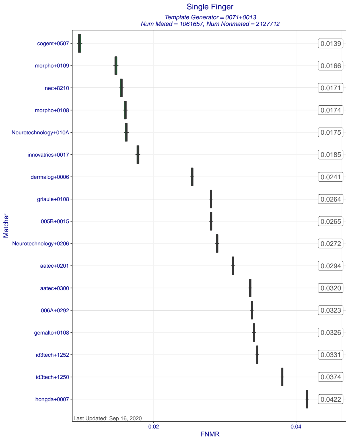
Figure 5: Single Finger FNMRs at FMR=0.0001 when MINEX III compliant matchers compare templates created by template generator 0071+0013. Each box represents uncertainty about the true FNMR. The box edges mark the 50% confidence intervals while the whiskers mark the 90% confidence intervals. The numbers on the right show the actual computed FNMRs.
