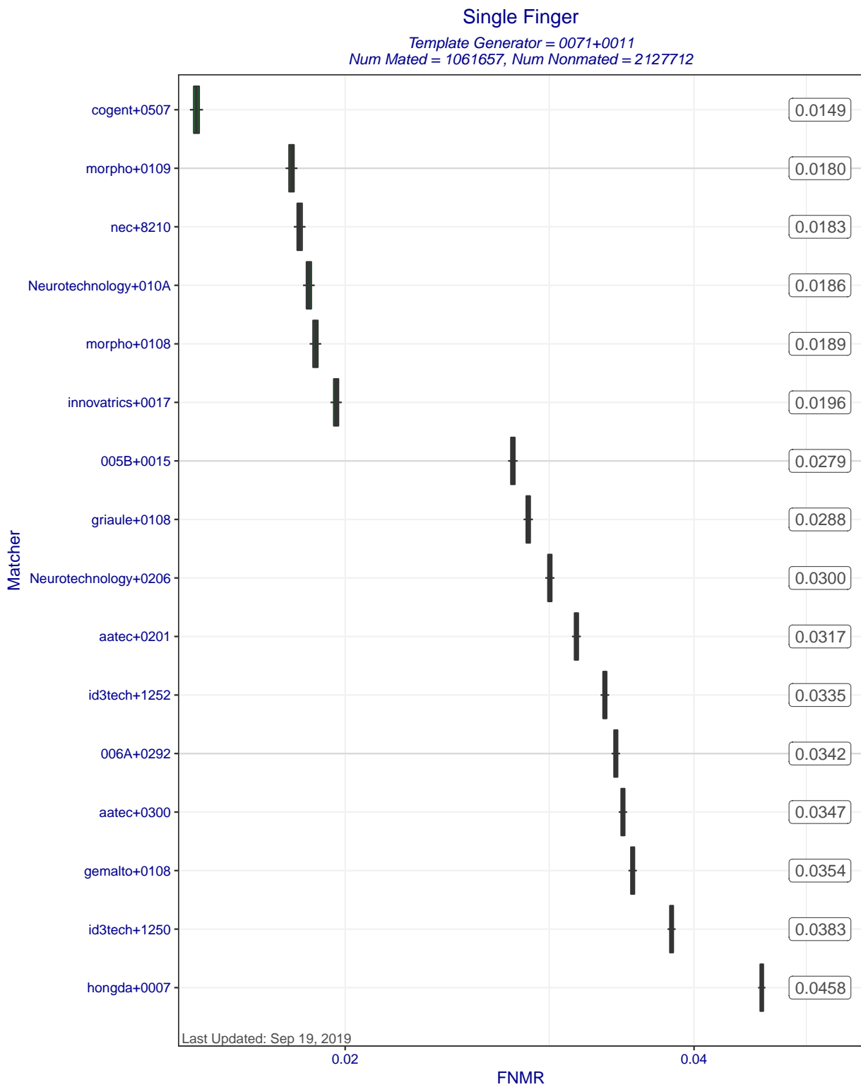
Figure 5: Single Finger FNMRs at FMR=0.0001 when MINEX III compliant matchers compare templates created by template generator 0071+0011. Each box represents uncertainty about the true FNMR. The box edges mark the 50% confidence intervals while the whiskers mark the 90% confidence intervals. The numbers on the right show the actual computed FNMRs.
