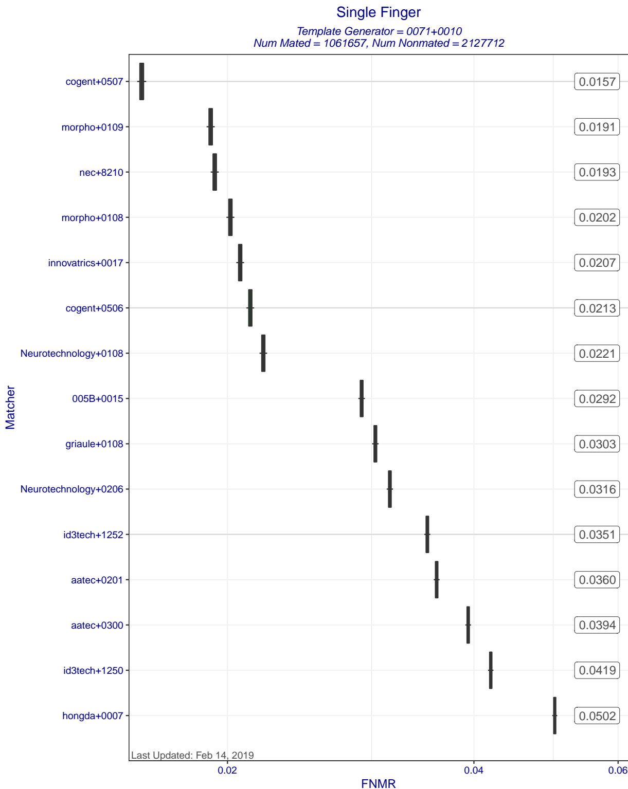
Figure 5: Single Finger FNMRs at FMR=0.0001 when MINEX III compliant matchers compare templates created by template generator 0071+0010. Each box represents uncertainty about the true FNMR. The box edges mark the 50% confidence intervals while the whiskers mark the 90% confidence intervals. The numbers on the right show the actual computed FNMRs.
