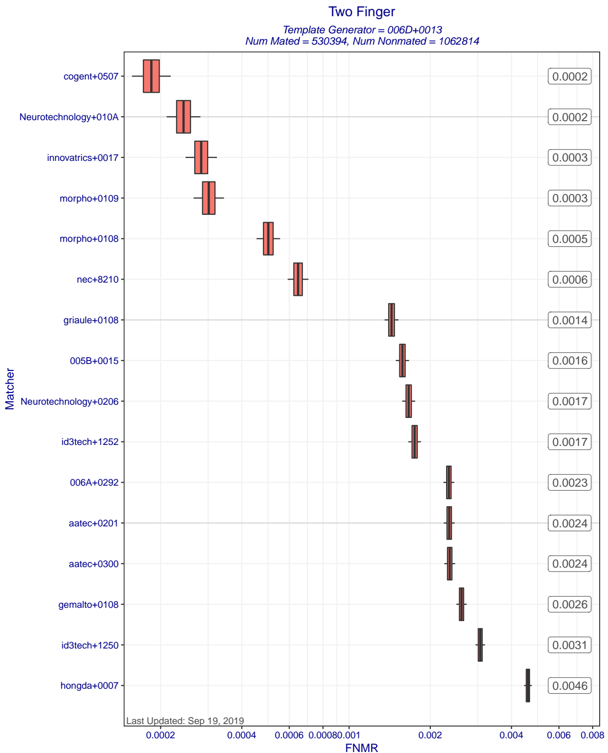
Figure 7: Two Finger FNMR at FMR=0.01 when different matchers compare templates created by template generator 006D+0013. Each box represents uncertainty about the true FNMR. The box edges mark the 50% confidence intervals while the whiskers mark the 90% confidence intervals. The numbers on the right show the actual computed FNMRs. Score-level fusion is achieved by averaging the scores for left and right index fingers.
