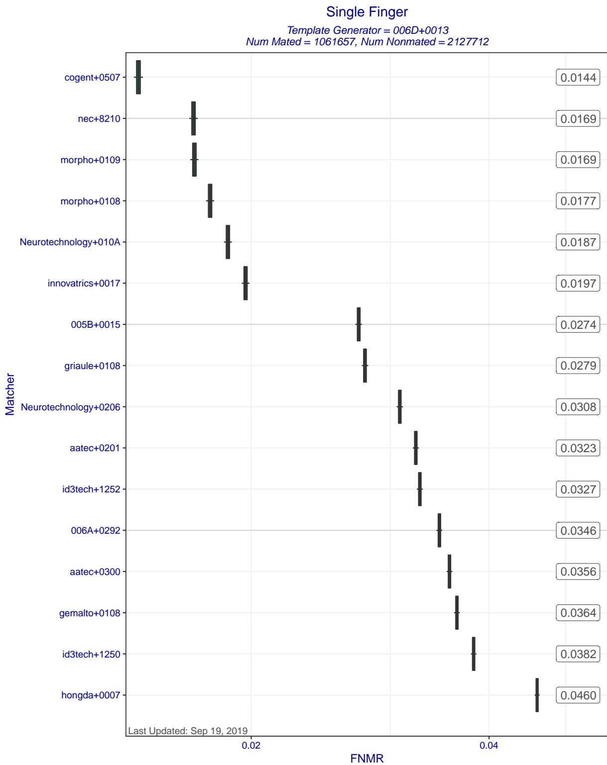
Figure 5: Single Finger FNMRs at FMR=0.0001 when MINEX III compliant matchers compare templates created by template generator 006D+0013. Each box represents uncertainty about the true FNMR. The box edges mark the 50% confidence intervals while the whiskers mark the 90% confidence intervals. The numbers on the right show the actual computed FNMRs.
