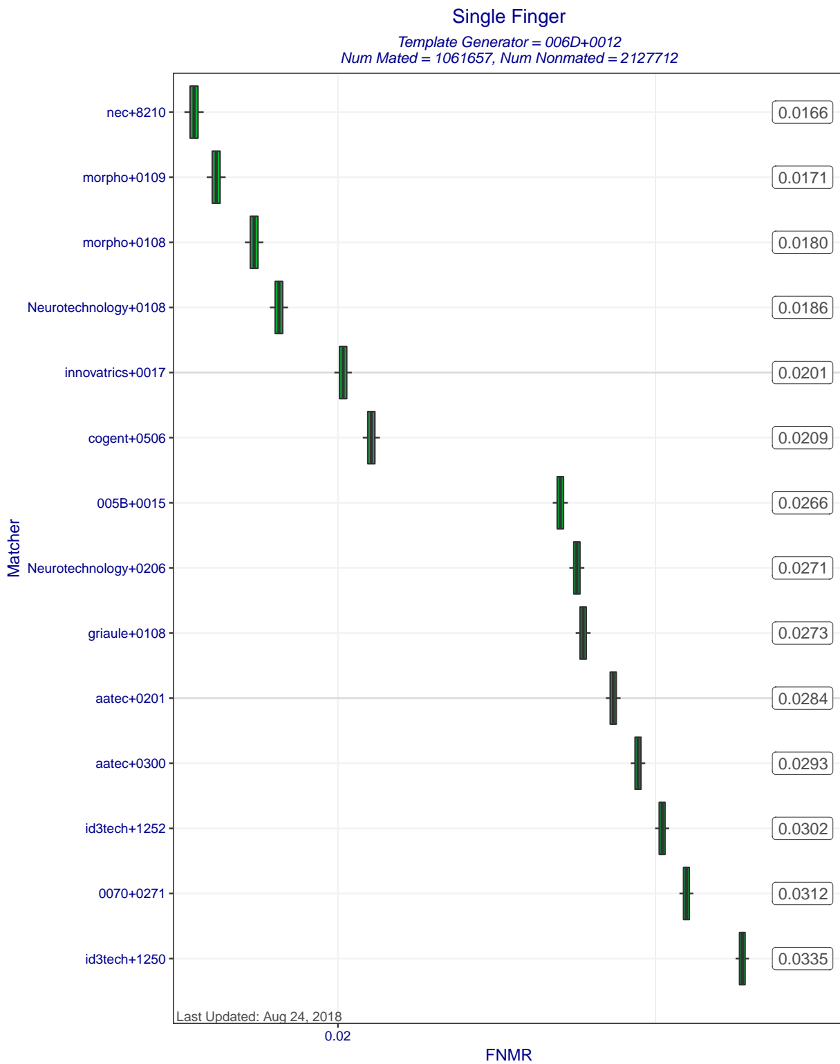
Figure 5: Single Finger FNMRs at FMR=0.0001 when MINEX III compliant matchers compare templates created by template generator 006D+0012. Each box represents uncertainty about the true FNMR. The box edges mark the 50% confidence intervals while the whiskers mark the 90% confidence intervals. The numbers on the right show the actual computed FNMRs.
