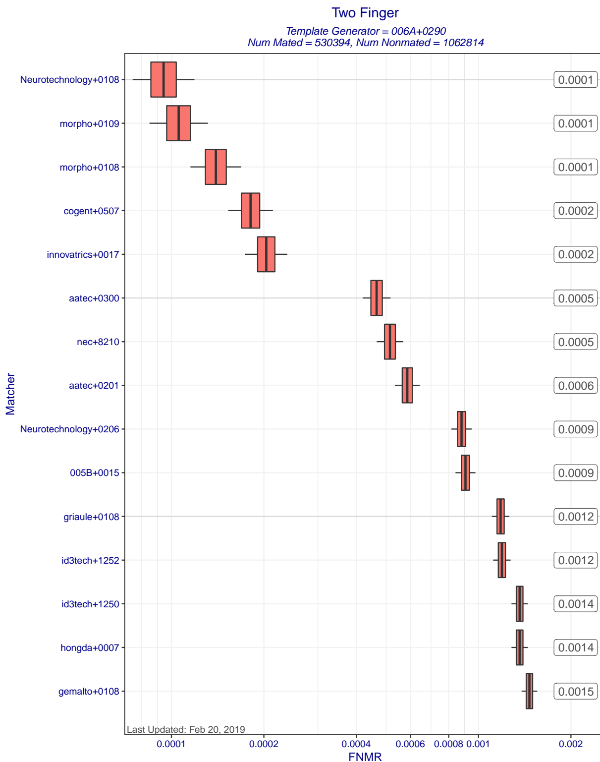
Figure 7: Two Finger FNMR at FMR=0.01 when different matchers compare templates created by template generator 006A+0290. Each box represents uncertainty about the true FNMR. The box edges mark the 50% confidence intervals while the whiskers mark the 90% confidence intervals. The numbers on the right show the actual computed FNMRs. Score-level fusion is achieved by averaging the scores for left and right index fingers.
