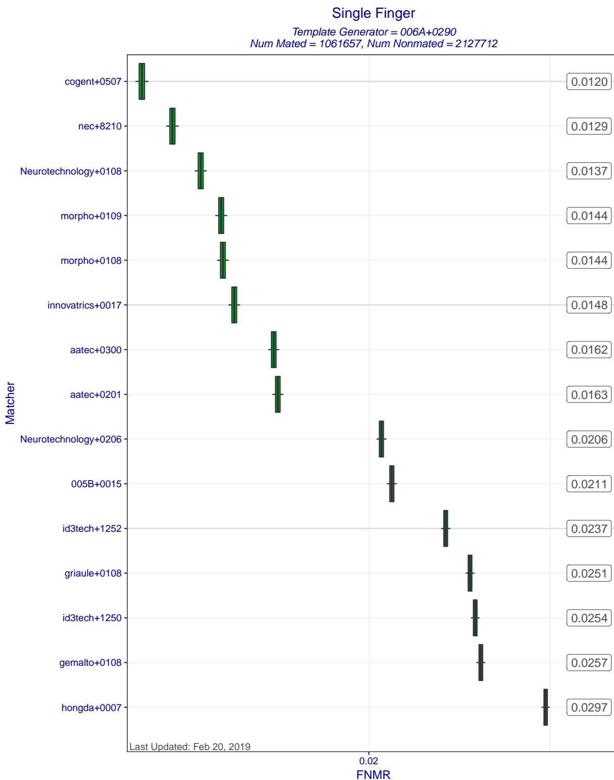
Figure 5: Single Finger FNMRs at FMR=0.0001 when MINEX III compliant matchers compare templates created by template generator 006A+0290. Each box represents uncertainty about the true FNMR. The box edges mark the 50% confidence intervals while the whiskers mark the 90% confidence intervals. The numbers on the right show the actual computed FNMRs.
