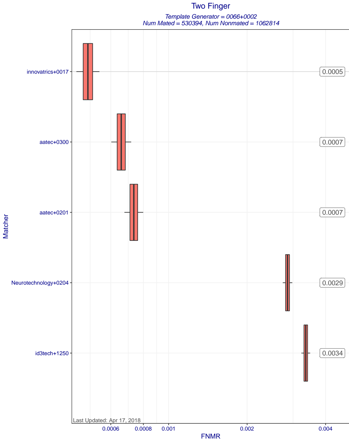
Figure 7: Two Finger FNMR at FMR=0.01 when different matchers compare templates created by template generator 0066+0002. Each box represents uncertainty about the true FNMR. The box edges mark the 50% confidence intervals while the whiskers mark the 90% confidence intervals. The numbers on the right show the actual computed FNMRs. Score-level fusion is achieved by averaging the scores for left and right index fingers.
