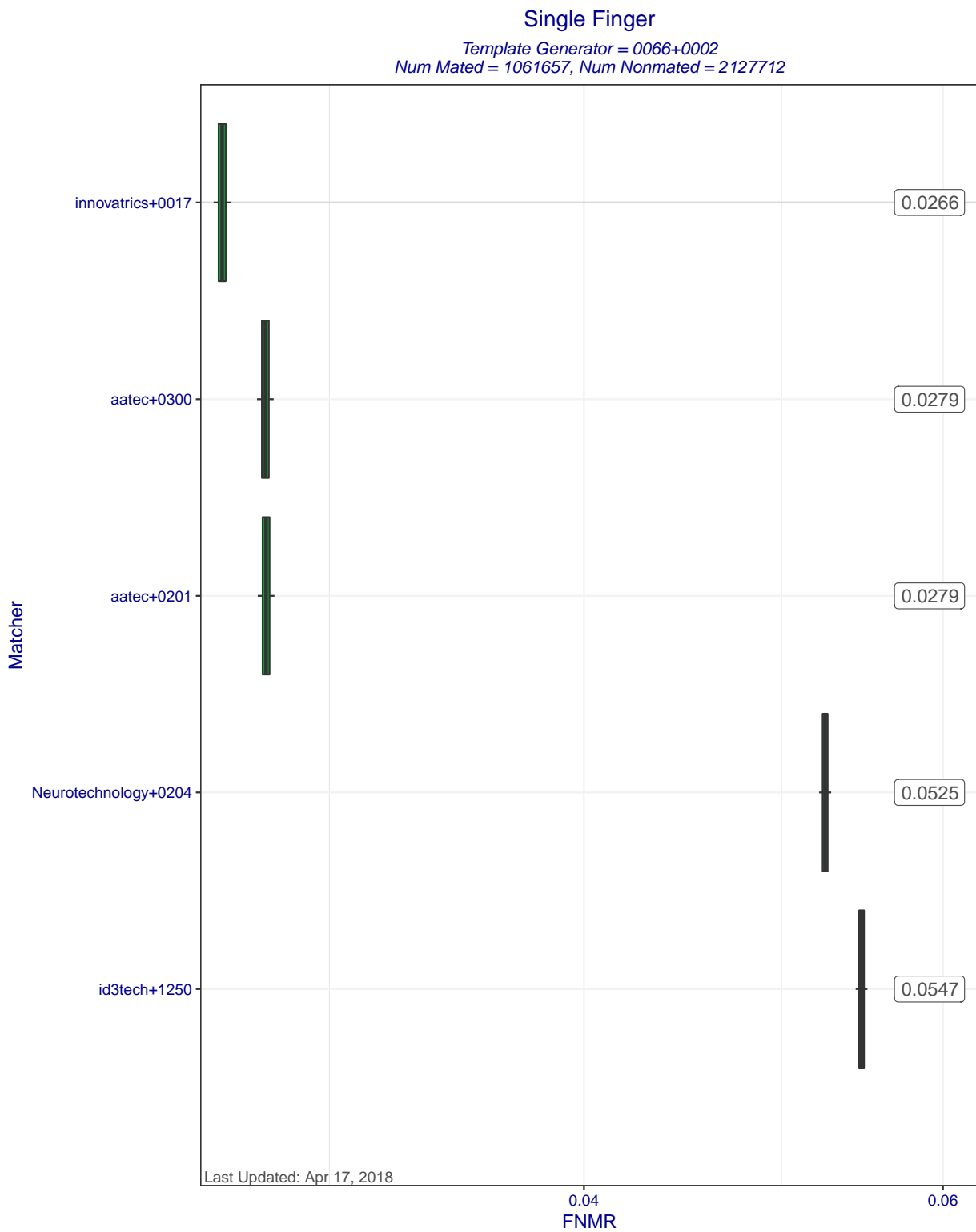
Figure 5: Single Finger FNMRs at FMR=0.0001 when MINEX III compliant matchers compare templates created by template generator 0066+0002. Each box represents uncertainty about the true FNMR. The box edges mark the 50% confidence intervals while the whiskers mark the 90% confidence intervals. The numbers on the right show the actual computed FNMRs.
