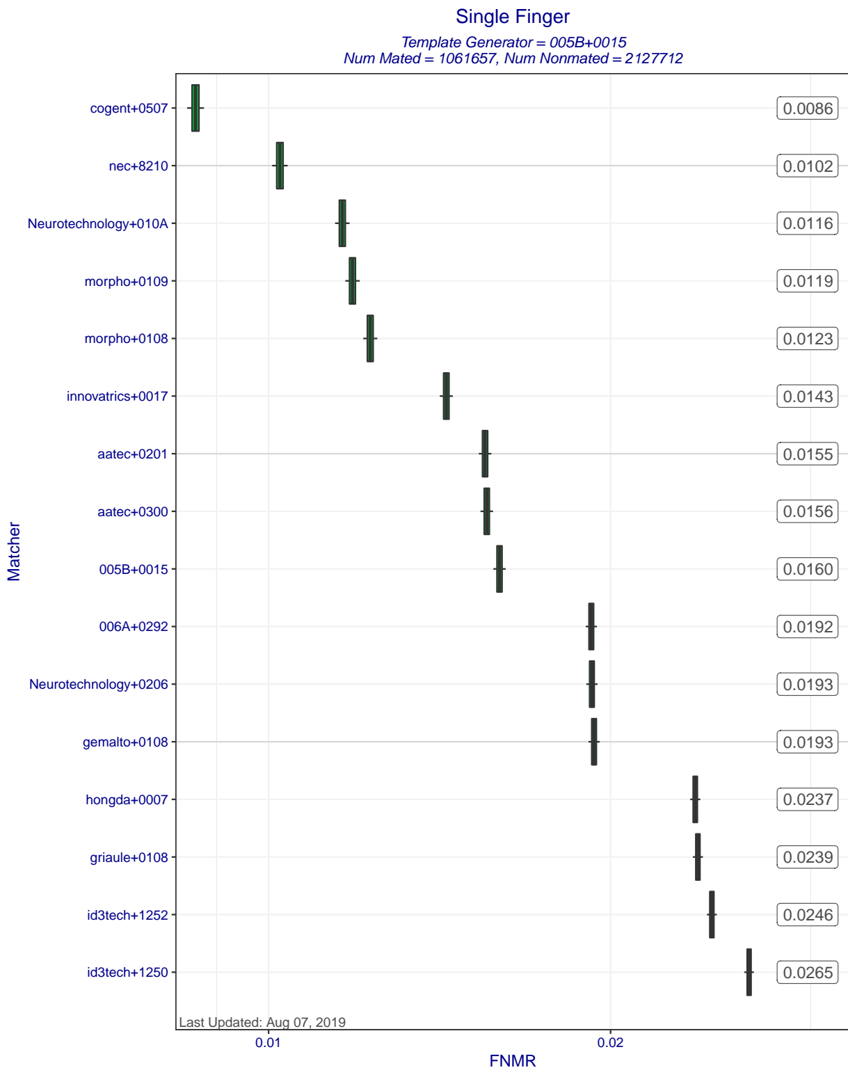
Figure 5: Single Finger FNMRs at FMR=0.0001 when MINEX III compliant matchers compare templates created by template generator 005B+0015. Each box represents uncertainty about the true FNMR. The box edges mark the 50% confidence intervals while the whiskers mark the 90% confidence intervals. The numbers on the right show the actual computed FNMRs.
