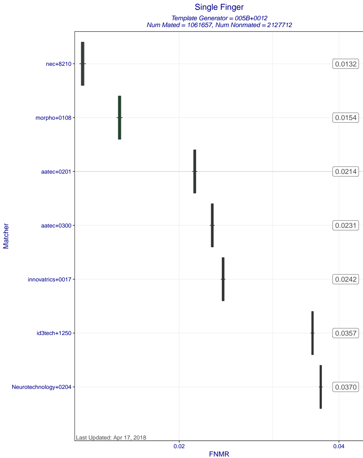
Figure 5: Single Finger FNMRs at FMR=0.0001 when MINEX III compliant matchers compare templates created by template generator 005B+0012. Each box represents uncertainty about the true FNMR. The box edges mark the 50% confidence intervals while the whiskers mark the 90% confidence intervals. The numbers on the right show the actual computed FNMRs.
