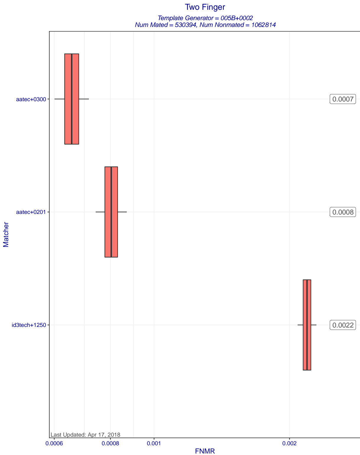
Figure 7: Two Finger FNMR at FMR=0.01 when different matchers compare templates created by template generator 005B+0002. Each box represents uncertainty about the true FNMR. The box edges mark the 50% confidence intervals while the whiskers mark the 90% confidence intervals. The numbers on the right show the actual computed FNMRs. Score-level fusion is achieved by averaging the scores for left and right index fingers.
