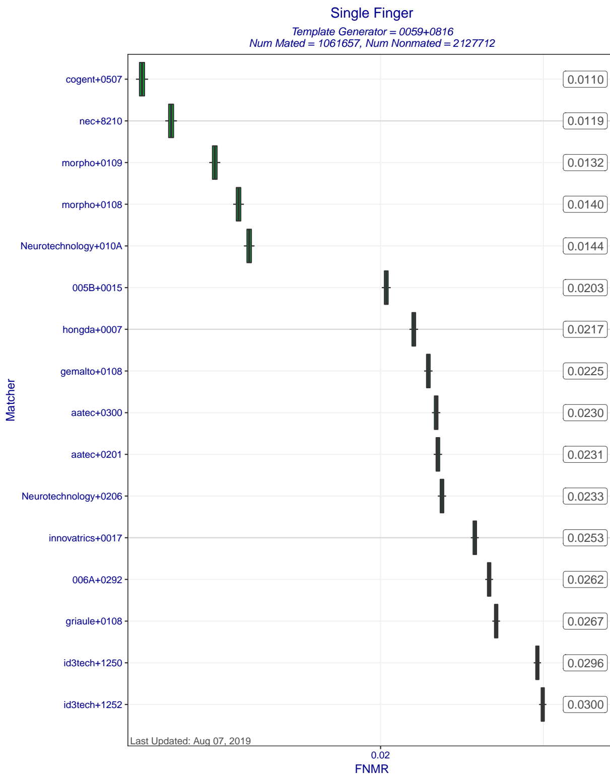
Figure 5: Single Finger FNMRs at FMR=0.0001 when MINEX III compliant matchers compare templates created by template generator 0059+0816. Each box represents uncertainty about the true FNMR. The box edges mark the 50% confidence intervals while the whiskers mark the 90% confidence intervals. The numbers on the right show the actual computed FNMRs.
