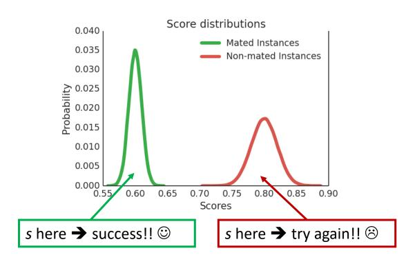
s can be the dissimilarity score of the system or any other dissimilarity score, such as values extracted from partial decoding in fuzzy schemes
