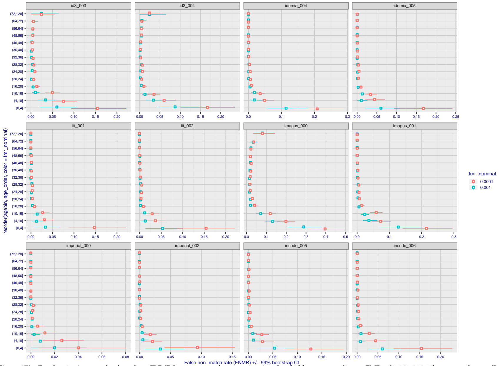
Figure 173: For the visa images, the dots show FNMR by age group for two operating thresholds corresponding to FMR = \{0.001, 0.0001\} computed over all on the order of 10^{10} impostor scores. The FMR in each bin will vary also - see subsequent impostor heatmaps in sec. 3.6.2. Given a pair of face images taken at different times, we assign the comparison to the bin that is the arithmetic average of the subject's ages. This plot shows only the effect of age, not ageing. The number of comparisons in each bin is generally in the thousands, however the first and last bins are computed over 149 and 124 respectively. The error rates in some (adult) cases are zero, and in others the DET is flat so the error rates at the two thresholds are identical. The lines span 1% and 99% of bootstrap replicated FNMR estimates.
