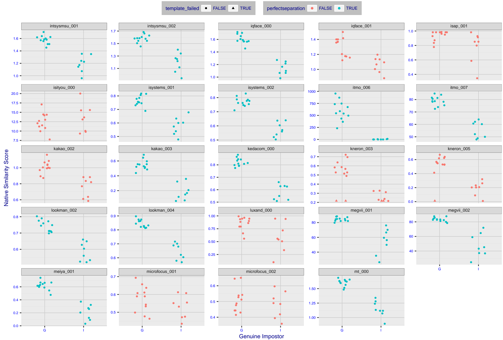
Figure 8: The Figure shows, in blue, algorithms that correctly separate the 12 genuine and 8 impostor pairs used in the May 2018 paper Face recognition accuracy of forensic examiners, superrecognizers, and face recognition algorithms (Phillips et al. [1]) . In red are algorithms that are imperfect. Some algorithms fail only because they failed to make a template e.g. due to face detection failure (shown as a triangle). Others fail because the pairs were selected for that study because they had been difficult for three leading algorithms used in FRVT 2006. Caution: Given the small sample size (n=20) the figure may change substantially if larger or different sets were used. The images can be downloaded from the Supplemental Information page provided with that publication.
