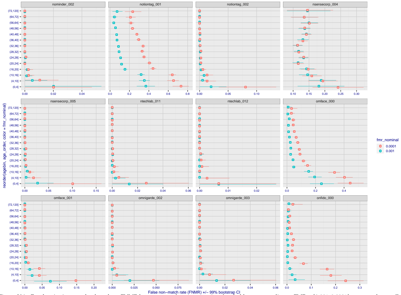
Figure 396: For the visa images, the dots show FNMR by age group for two operating thresholds corresponding to FMR = \{0.001, 0.0001\} computed over all on the order of 10^{10} impostor scores. The FMR in each bin will vary also - see subsequent impostor heatmaps in sec. 3.6.2. Given a pair of face images taken at different times, we assign the comparison to the bin that is the arithmetic average of the subject's ages. This plot shows only the effect of age, not ageing. The number of comparisons in each bin is generally in the thousands, however the first and last bins are computed over 149 and 124 respectively. The error rates in some (adult) cases are zero, and in others the DET is flat so the error rates at the two thresholds are identical. The lines span 1% and 99% of bootstrap replicated FNMR estimates.
