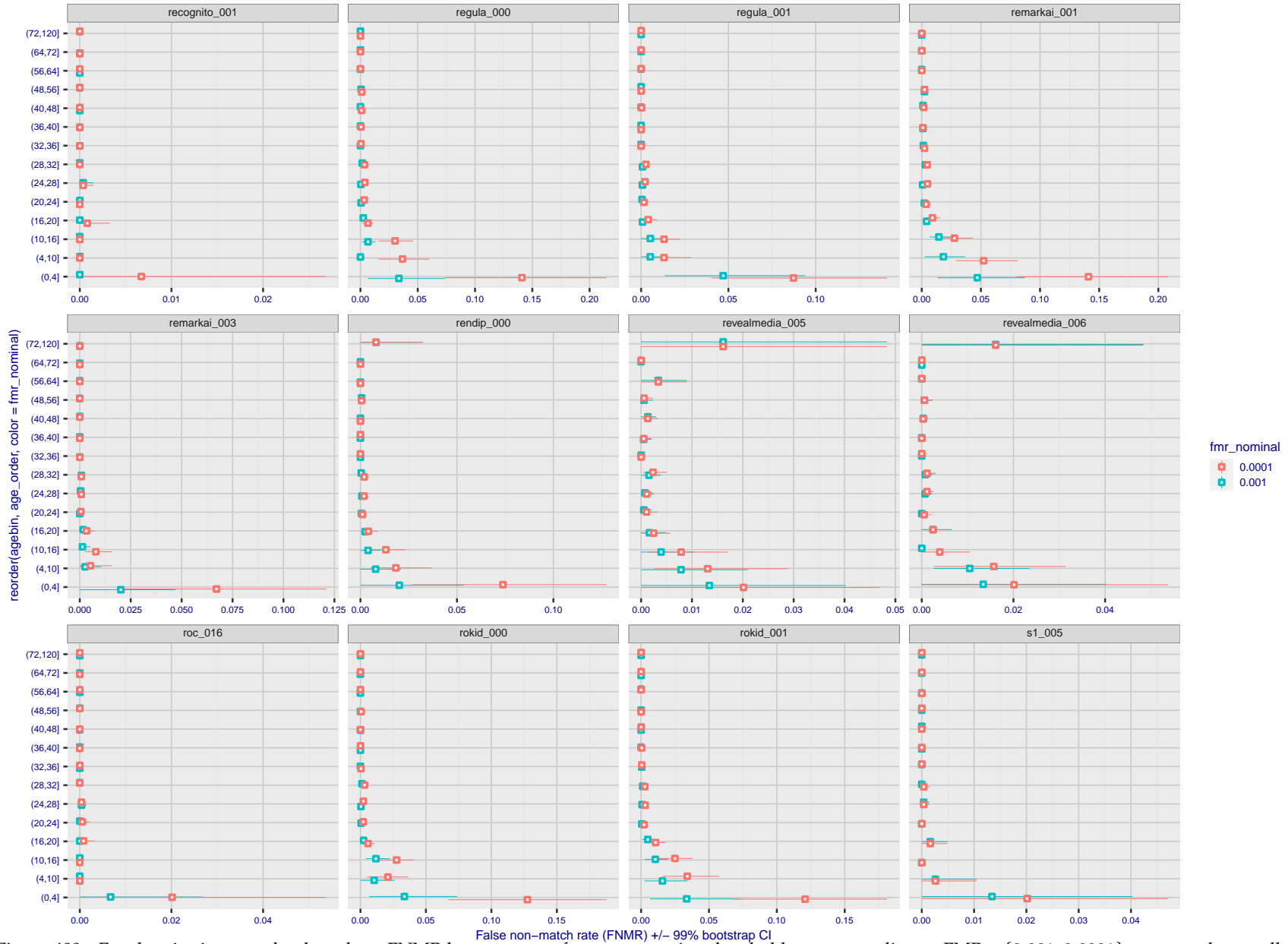
Figure 400: For the visa images, the dots show FNMR by age group for two operating thresholds corresponding to FMR = \{0.001, 0.0001\} computed over all on the order of 10^{10} impostor scores. The FMR in each bin will vary also - see subsequent impostor heatmaps in sec. 3.6.2. Given a pair of face images taken at different times, we assign the comparison to the bin that is the arithmetic average of the subject's ages. This plot shows only the effect of age, not ageing. The number of comparisons in each bin is generally in the thousands, however the first and last bins are computed over 149 and 124 respectively. The error rates in some (adult) cases are zero, and in others the DET is flat so the error rates at the two thresholds are identical. The lines span 1% and 99% of bootstrap replicated FNMR estimates.
