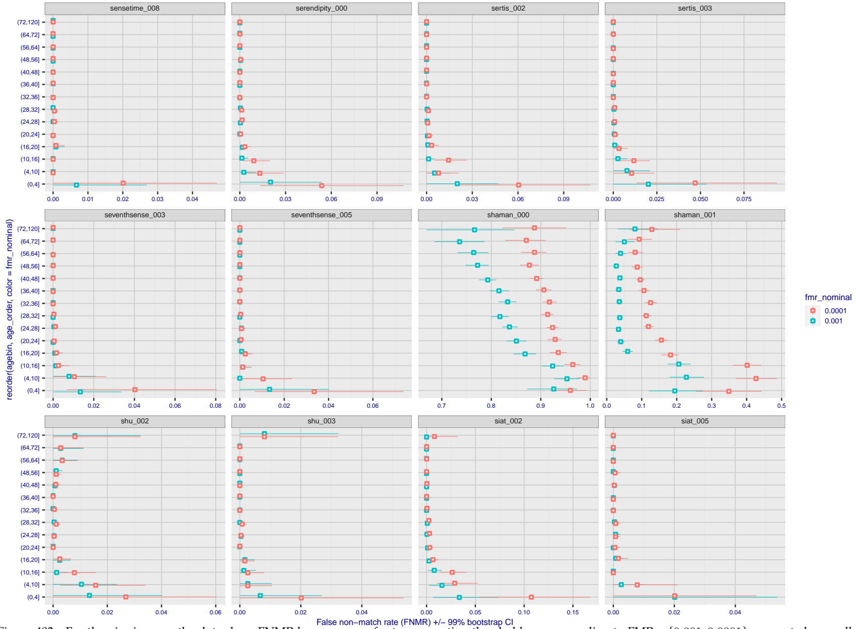
Figure 402: For the visa images, the dots show FNMR by age group for two operating thresholds corresponding to FMR = \{0.001, 0.0001\} computed over all on the order of 10^{10} impostor scores. The FMR in each bin will vary also - see subsequent impostor heatmaps in sec. 3.6.2. Given a pair of face images taken at different times, we assign the comparison to the bin that is the arithmetic average of the subject's ages. This plot shows only the effect of age, not ageing. The number of comparisons in each bin is generally in the thousands, however the first and last bins are computed over 149 and 124 respectively. The error rates in some (adult) cases are zero, and in others the DET is flat so the error rates at the two thresholds are identical. The lines span 1% and 99% of bootstrap replicated FNMR estimates.
