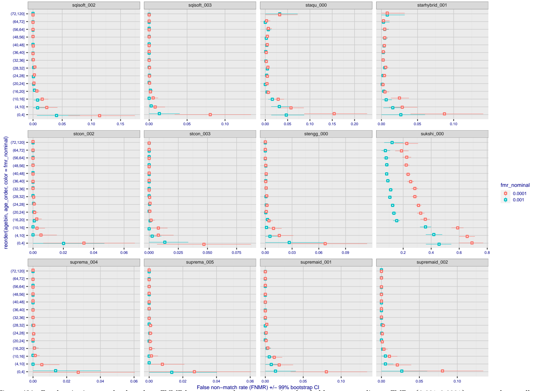
Figure 404: For the visa images, the dots show FNMR by age group for two operating thresholds corresponding to FMR = \{0.001, 0.0001\} computed over all on the order of 10^{10} impostor scores. The FMR in each bin will vary also - see subsequent impostor heatmaps in sec. 3.6.2. Given a pair of face images taken at different times, we assign the comparison to the bin that is the arithmetic average of the subject's ages. This plot shows only the effect of age, not ageing. The number of comparisons in each bin is generally in the thousands, however the first and last bins are computed over 149 and 124 respectively. The error rates in some (adult) cases are zero, and in others the DET is flat so the error rates at the two thresholds are identical. The lines span 1% and 99% of bootstrap replicated FNMR estimates.
