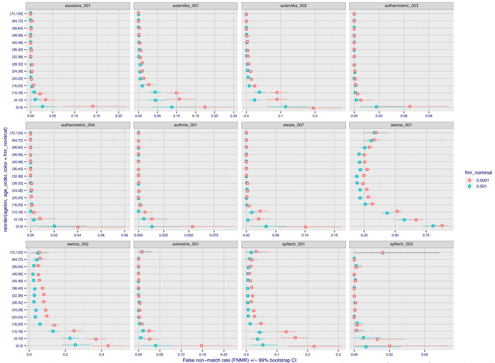
Figure 373: For the visa images, the dots show FNMR by age group for two operating thresholds corresponding to FMR = \{0.001, 0.0001\} computed over all on the order of 10^{10} impostor scores. The FMR in each bin will vary also - see subsequent impostor heatmaps in sec. 3.6.2. Given a pair of face images taken at different times, we assign the comparison to the bin that is the arithmetic average of the subject's ages. This plot shows only the effect of age, not ageing. The number of comparisons in each bin is generally in the thousands, however the first and last bins are computed over 149 and 124 respectively. The error rates in some (adult) cases are zero, and in others the DET is flat so the error rates at the two thresholds are identical. The lines span 1% and 99% of bootstrap replicated FNMR estimates.
