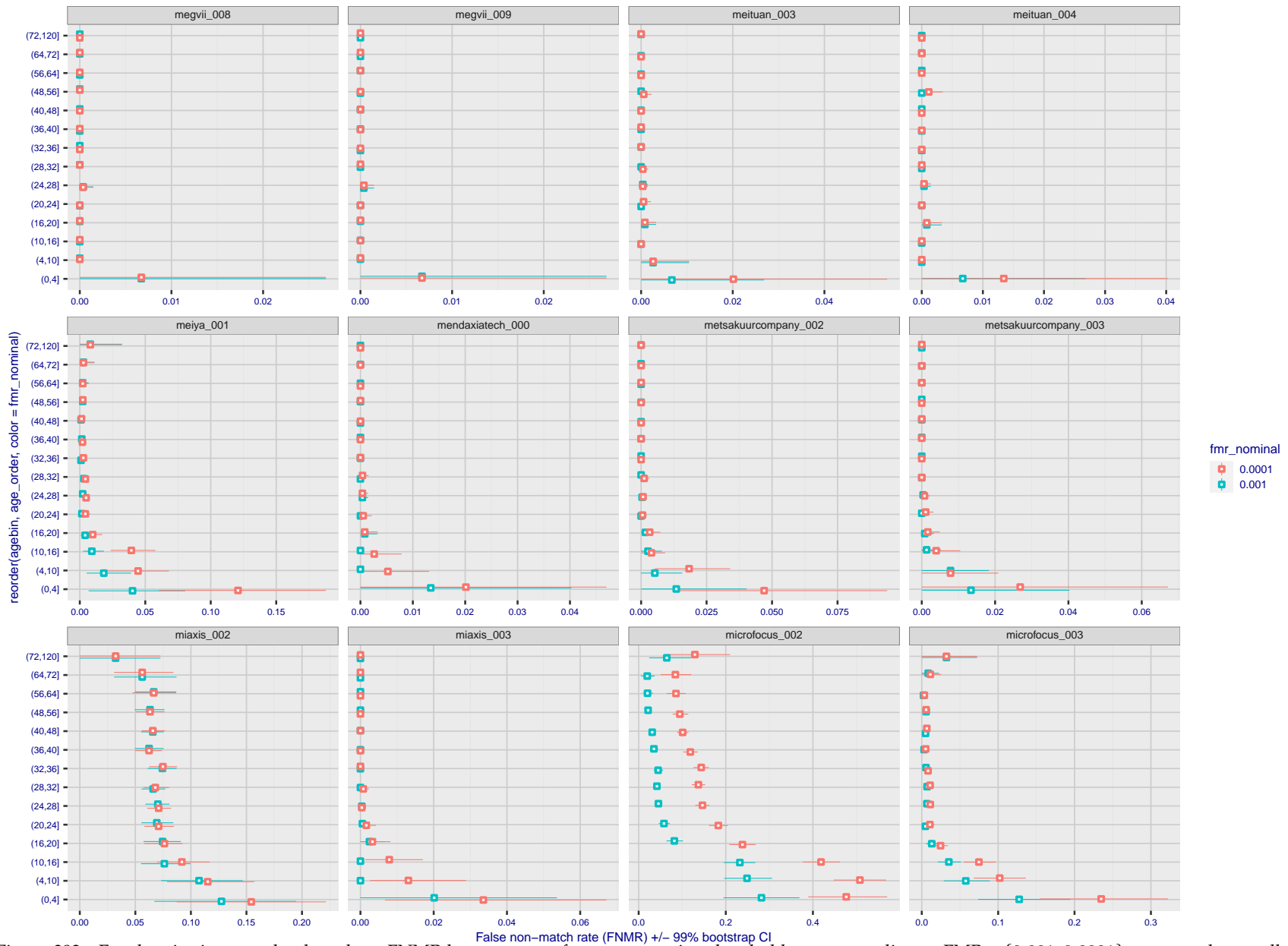
Figure 393: For the visa images, the dots show FNMR by age group for two operating thresholds corresponding to FMR = \{0.001, 0.0001\} computed over all on the order of 10^{10} impostor scores. The FMR in each bin will vary also - see subsequent impostor heatmaps in sec. 3.6.2. Given a pair of face images taken at different times, we assign the comparison to the bin that is the arithmetic average of the subject's ages. This plot shows only the effect of age, not ageing. The number of comparisons in each bin is generally in the thousands, however the first and last bins are computed over 149 and 124 respectively. The error rates in some (adult) cases are zero, and in others the DET is flat so the error rates at the two thresholds are identical. The lines span 1% and 99% of bootstrap replicated FNMR estimates.
