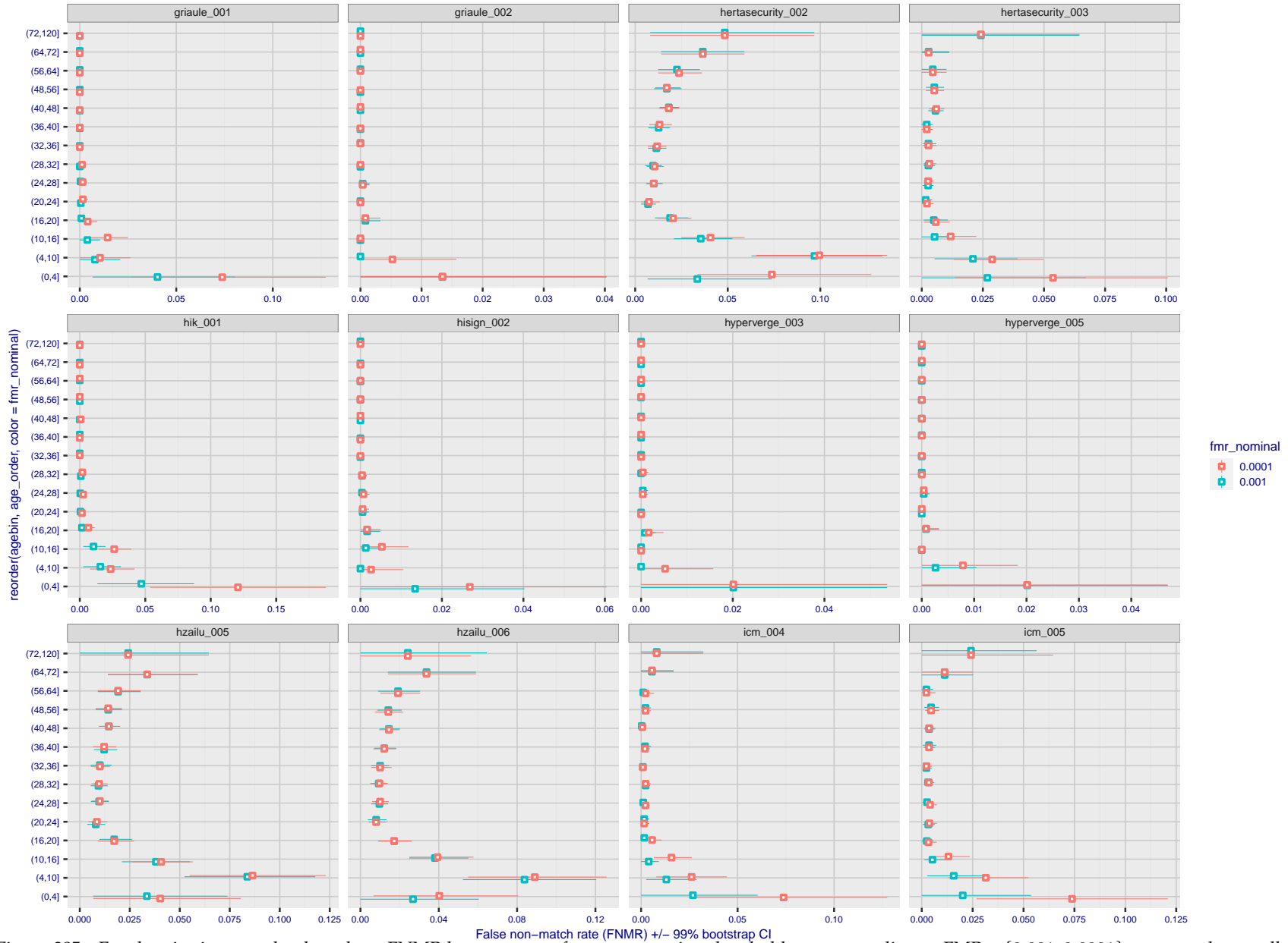
Figure 385: For the visa images, the dots show FNMR by age group for two operating thresholds corresponding to FMR = \{0.001, 0.0001\} computed over all on the order of 10^{10} impostor scores. The FMR in each bin will vary also - see subsequent impostor heatmaps in sec. 3.6.2. Given a pair of face images taken at different times, we assign the comparison to the bin that is the arithmetic average of the subject's ages. This plot shows only the effect of age, not ageing. The number of comparisons in each bin is generally in the thousands, however the first and last bins are computed over 149 and 124 respectively. The error rates in some (adult) cases are zero, and in others the DET is flat so the error rates at the two thresholds are identical. The lines span 1% and 99% of bootstrap replicated FNMR estimates.
